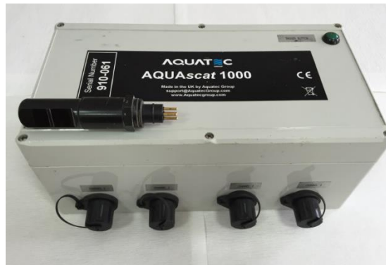
Figure 1. The AQUAscat-L (Aquatec Group) device and seapoint turbidity meter sensor
