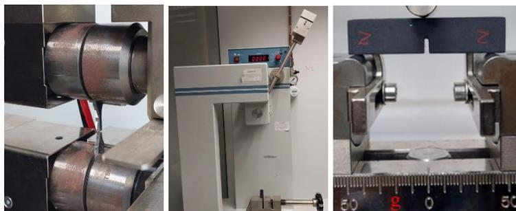
Figure 3. Specimens under tensile, Impact and SENB tests
