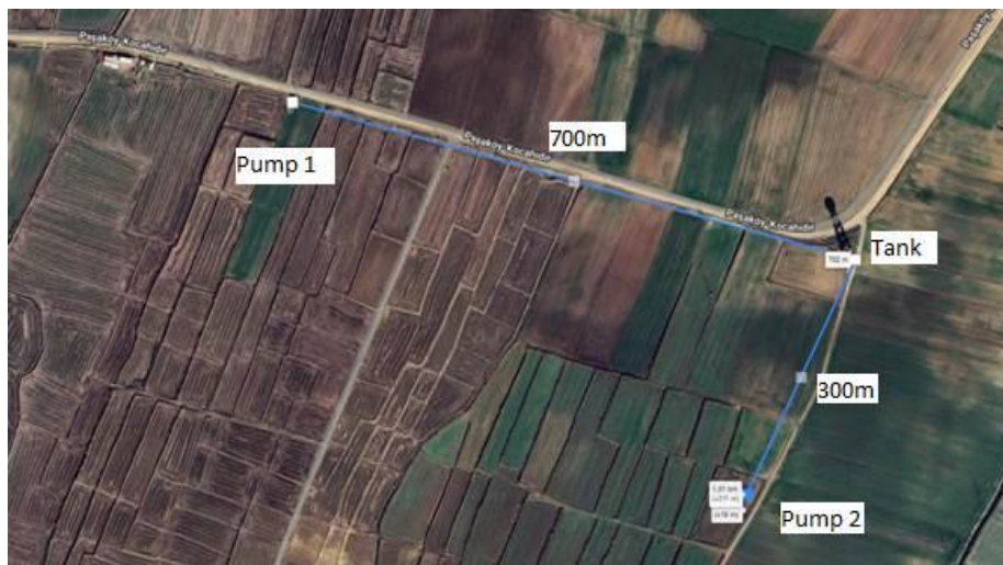
Figure 2. Locations of the pumps and the water tank
