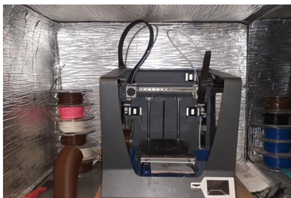
Figure 2. Printer used for the production of polymer gear wheels
