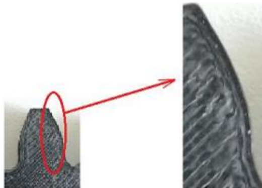
Figure 7. Specimen with wall thickness as 0.4 mm
