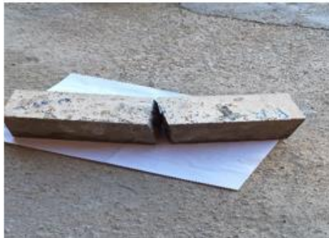
Figure12. Fragile failure at mid-span of the control SCCR specimen
