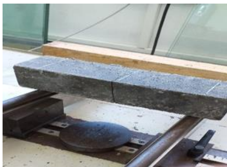
Figure 13. Fragile failure at mid-span of fiberized SCC specimen
