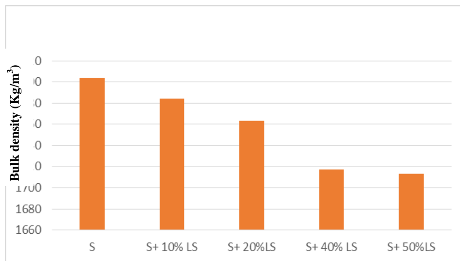
Figure 11. Bulk density of stabilized blocks with lightweight sand
