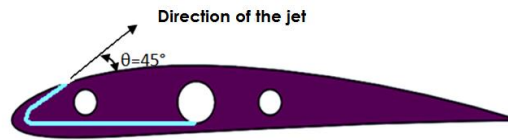
Figure 4. Sectional view showing the position of the blowing orifices on the model. The arrow indicates the jet direction as well as the tilting angle \theta of the blowing nozzles.
