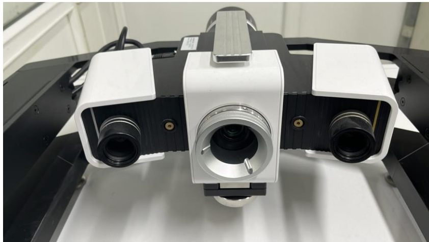
Figure 4. The check of dimensional accuracy of plastic products with 3D optical scanner
