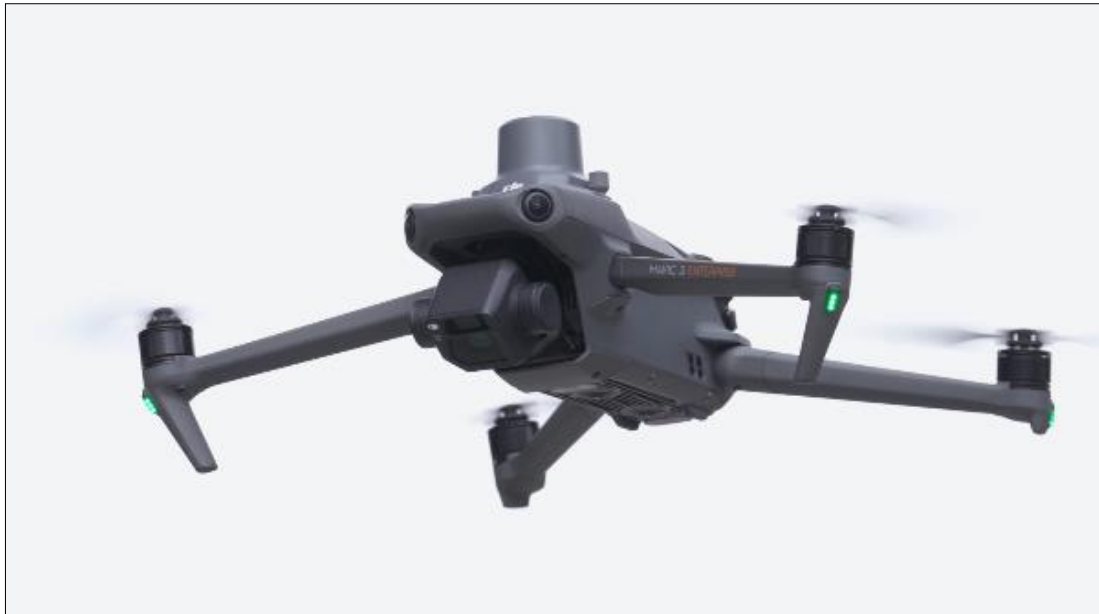
Figure 2. DJI Mavic 3 enterprise RTK (URL-7). The cylindrical apparatus on top of the UAV functions as the RTK unit.
