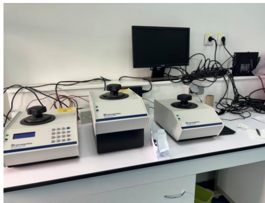
Figure 11. Overview of the helium pycnometer and its instrumentation
