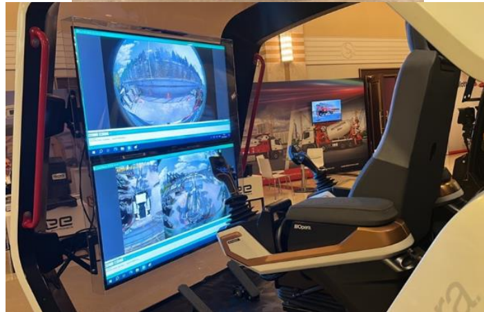
Figure 1. & Figure 2. The exterior and interior view of Hidromek opera, remote-control station.
