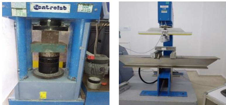
Figure 4. Compressive and flexural strength tests
