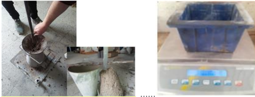
Figure 3. Fresh state tests: Slump test and bulk density.
