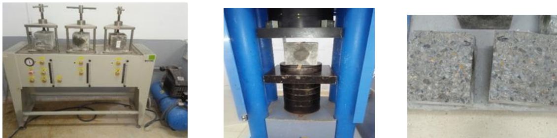
Figure 6. Water permeability test
