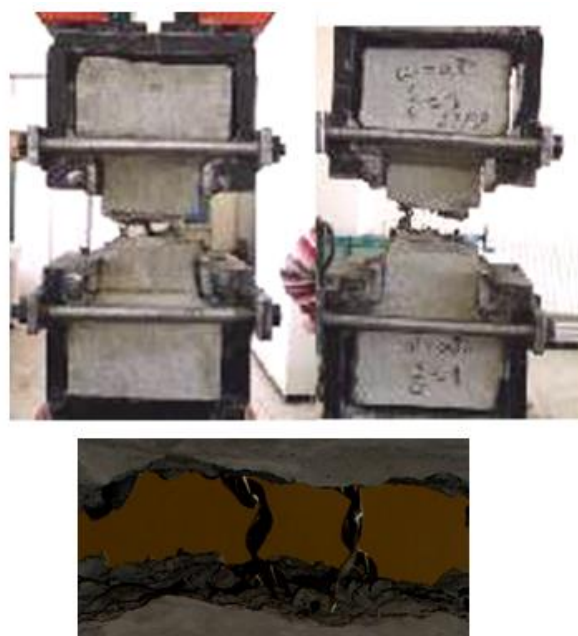
Figure 18. Failure mode of fibers in tension
