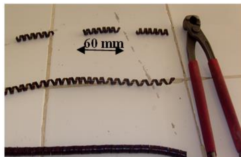
Figure 1. View of fibers in chips
