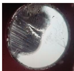
Figure 9a. Cutting a fiber well fixed in tool
