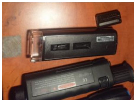
Figure 7a) Optical microscope used for fiber optic polishing quality investigation (video microscope n.d )
