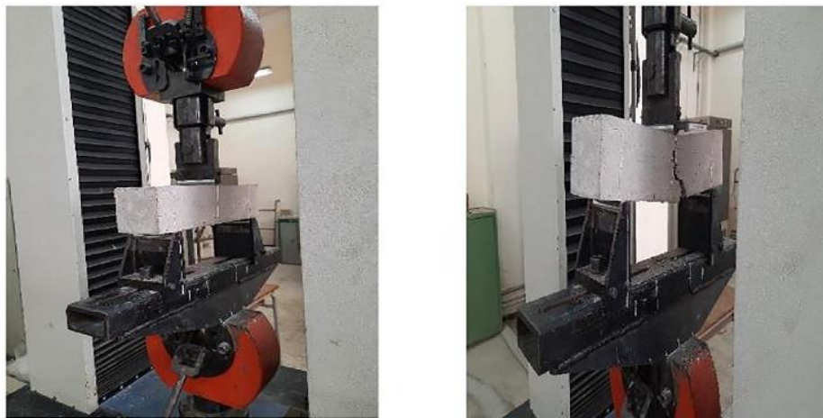
Figure 10. The setup of the three-point bending test
