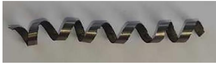
Figure 12. Fibers used L = 6 cm with 6 undulations
