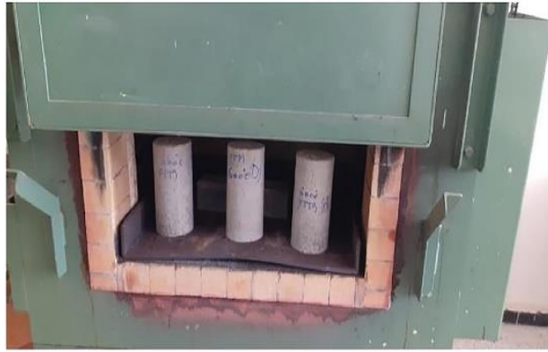
Figure 6. Arrangement of the test pieces inside the oven
