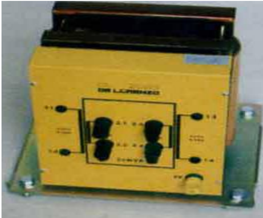
Figure 1. Real used transformer
