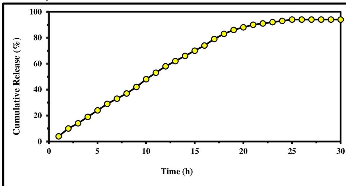
Figure 7. Cu+2 release in water from NaCMC-4 hydrogel
