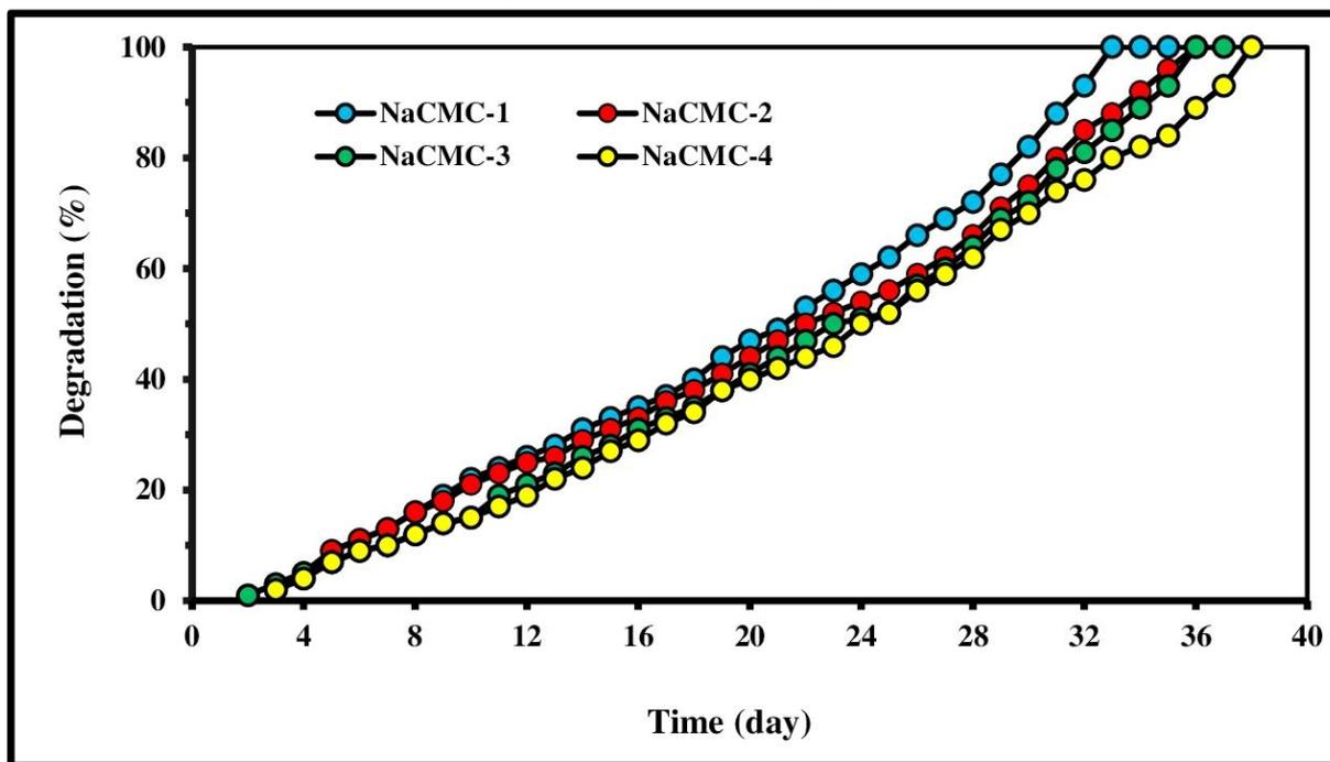
Figure 5. The degradation profiles of hydrogels at 30°C
