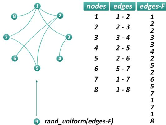
Figure 1. The computational method followed to achieve a BA network is illustrated. The new node (9) just joining the network chooses a node to connect from the flattened edges array (edges-F), with an index randomly generated from a uniform distribution. By the way, nodes have attachment probabilities proportional with their current degrees
