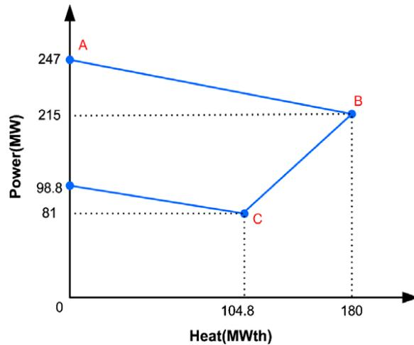
Figure 3. Feasible operation region for the cogeneration unit 2 for system1 and unit 5 for system2
