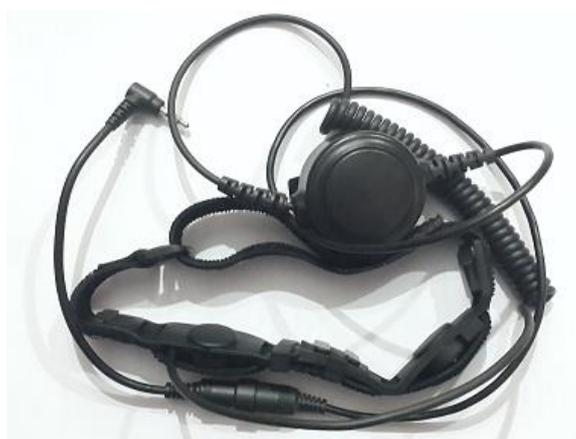
Figure 4. Throat microphone with two sensors
