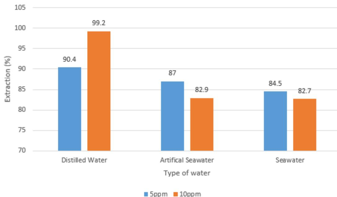
Figure 2. Comparison of percentage of cadmium metal extraction using 5.0 ppm and 10.0 ppm Cd (NO<sub>3</sub>)<sub>2</sub>
