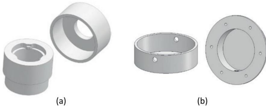
Figure 2. Specimen holders (a) for solids (b) for liquids
