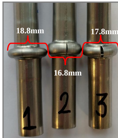
Figure 8. Samples with damaged or undamaged welded seams after expansion test
