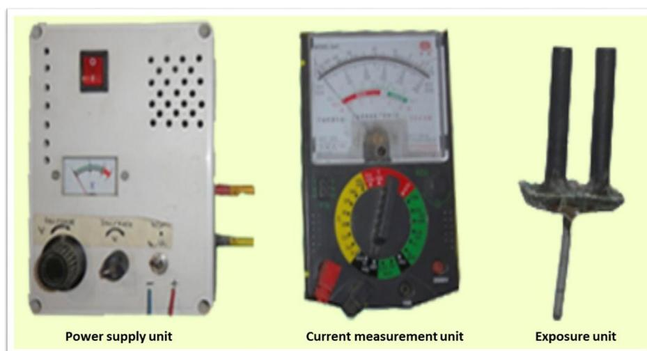
Image 2. Direct electrical current device
