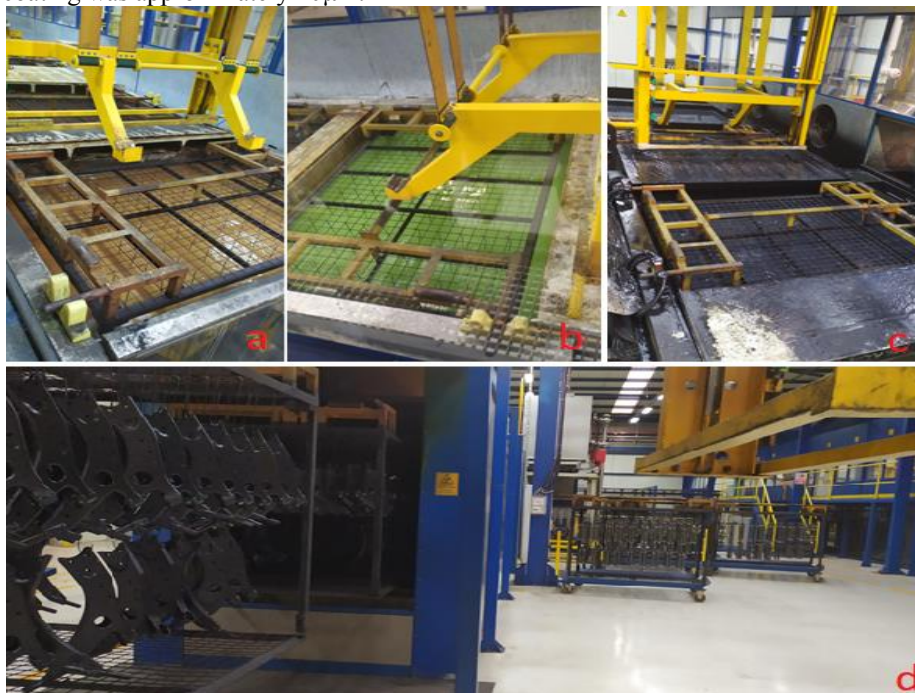
Figure 2. a) Surface cleaning, b) Surface preparation, c) Coating, d) Flash-off and oven
