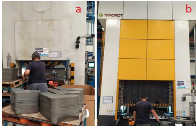
Figure 1. a) Template cutting press, b) Sheet forming press
