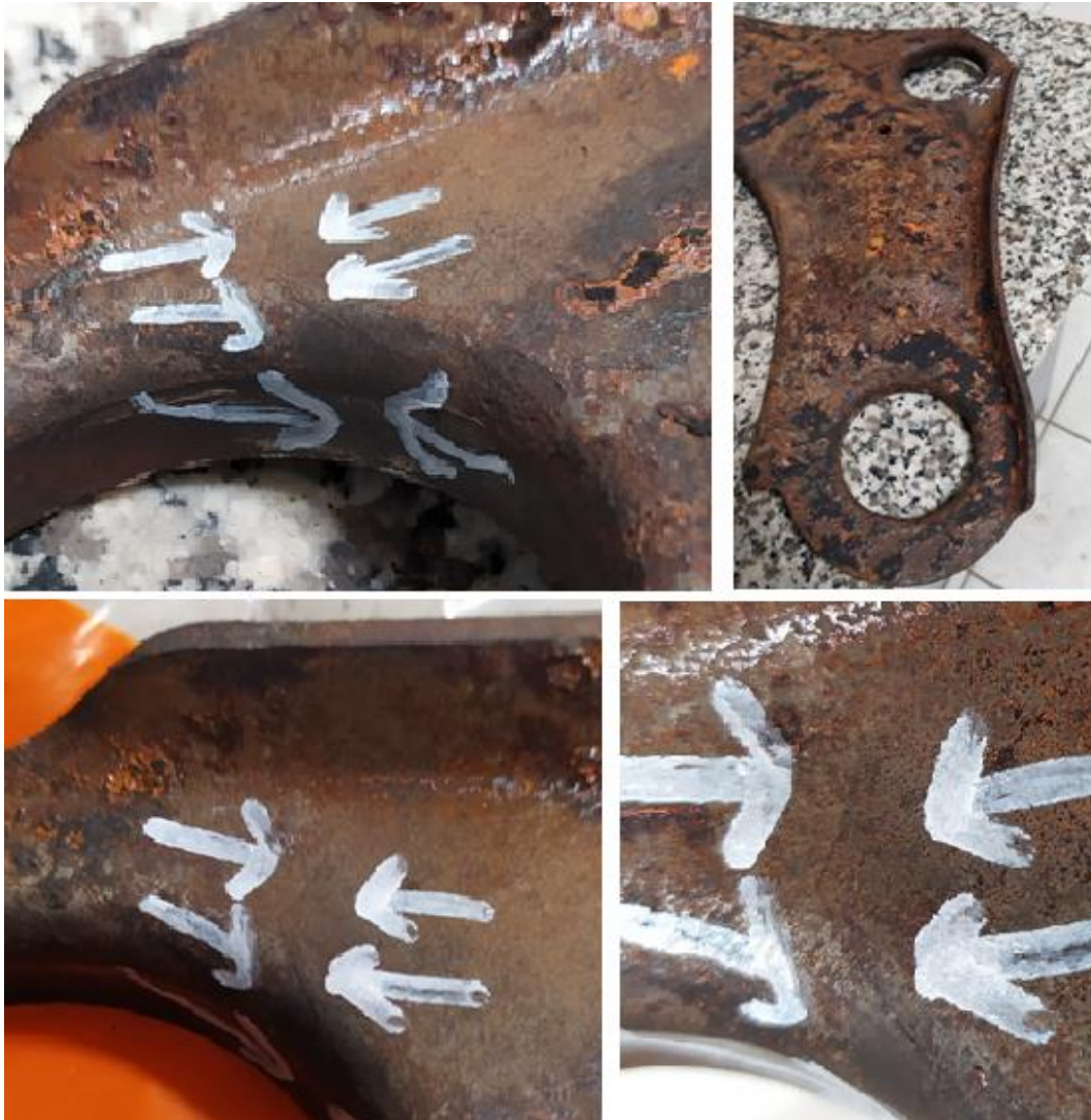
Figure 7. Crack regions on the uncoated parts after fatigue test
