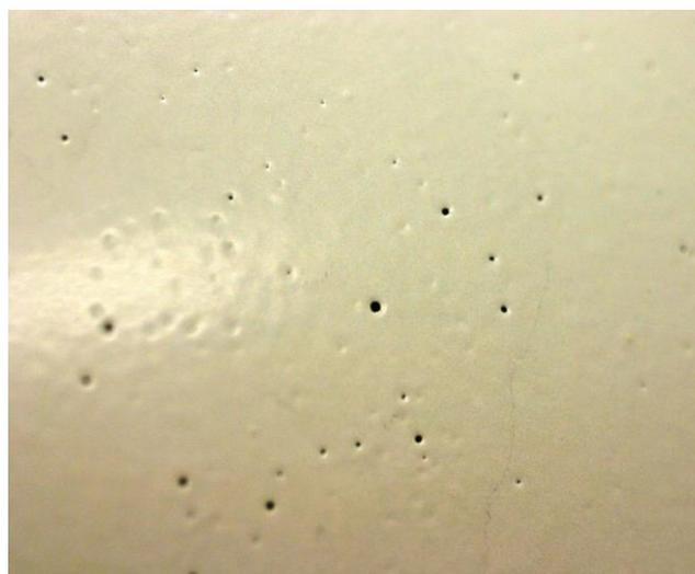
Figure 3. Pinhole defects after cataphoretic coating.
