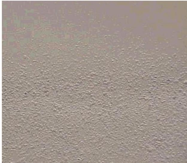
Figure 1. Dirt based defects after cataphoretic coating.
