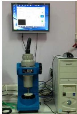
Figure 3. Dynamic Shear Rheometer test device
