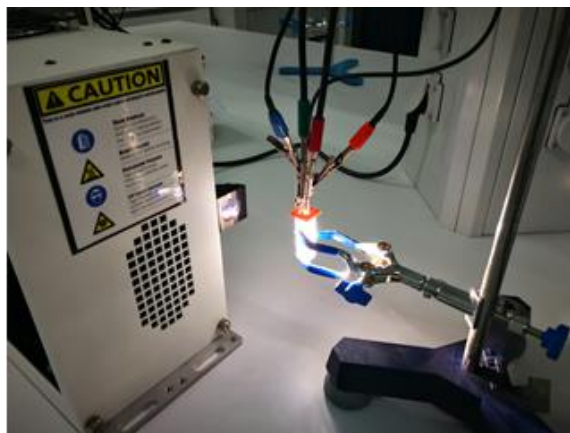
Figure 3. The photo-current measurements of CVD graphene - g-C 3 N 4 composites.
