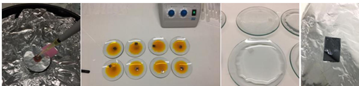
Figure 2. Cleaning and transfer processes of graphene after synthesis by CVD.
