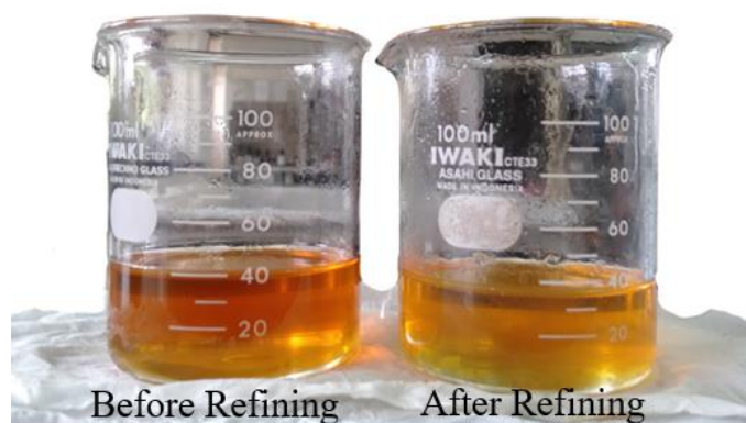
Figure 1. Discolouration of waste cooking oil in refining process.
