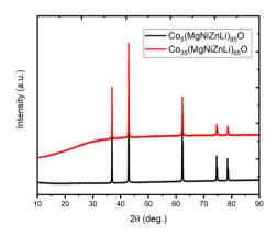
Figure 1. XRD patterns of the as-synthesized Co<sub>5</sub>(MgNiZnLi)<sub>95</sub>O and Co<sub>35</sub>(MgNiZnLi)<sub>65</sub>O HEOs.
