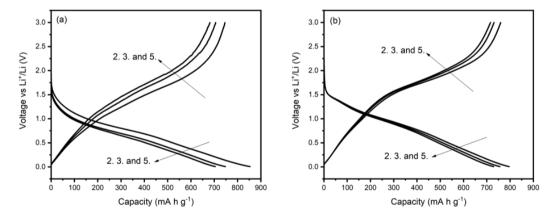
Figure 3. Discharge-charge curves of (a) Co<sub>5</sub>(MgNiZnLi)<sub>95</sub>O and (b) Co<sub>35</sub>(MgNiZnLi)<sub>65</sub>O anodes for the 2<sup>nd</sup>, 3<sup>rd</sup> and 5<sup>th</sup> cycles in the voltage range of 0.01-3.00 V at a current density of 100 mA g<sup>-1</sup>.
