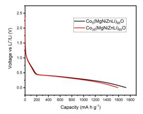
Figure 2. Initial discharge curves of  $Co_5(MgNiZnLi)_{95}O$  and  $Co_{35}(MgNiZnLi)_{65}O$  anodes at a current density of 100 mA g<sup>-1</sup>
