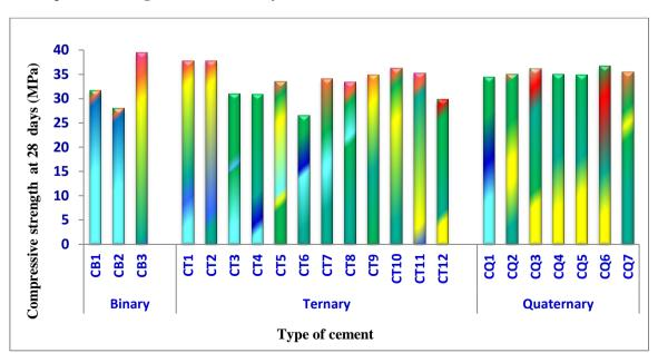
Figure 3. Variation of the compressive strength measured of the mortars at the age of 28 days.
