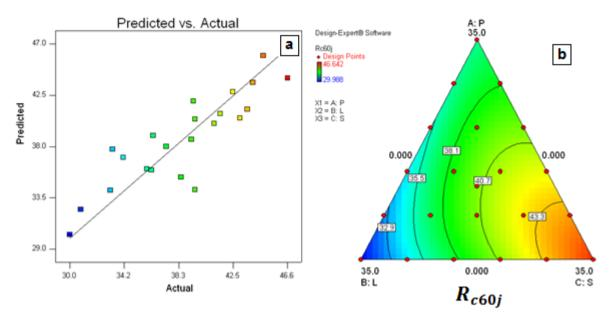
Figure 8. Compressive strength at 60 days a) Correlation between observed values and the model, b) Variation of compressive strength according to the model.
