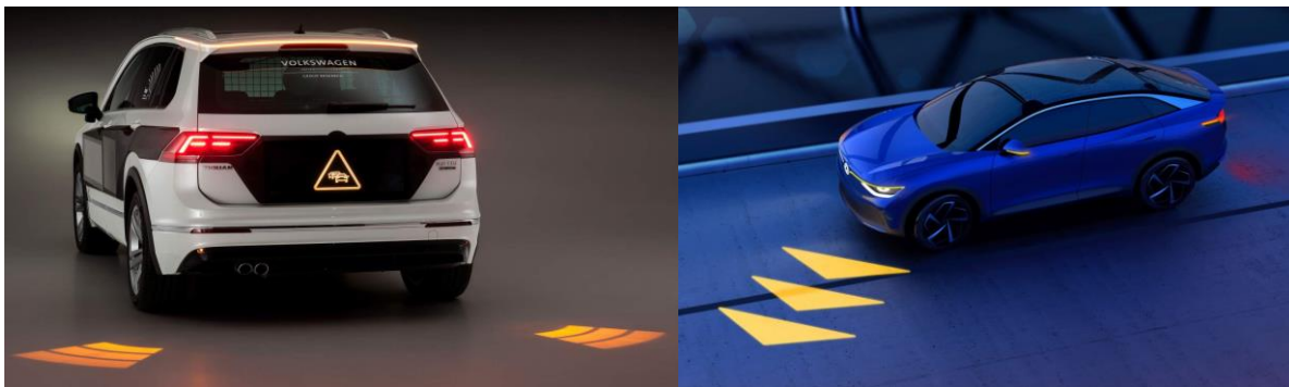
(a) Projection of signalling in tail light (Volkswagen, 2018) (b) Projection of signalling in front light (Blain, 2018) Figure 8. Projection function of signal lighting
