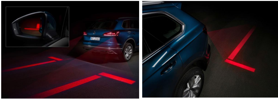
Figure 7. Optical park assist (Volkswagen, 2018)
