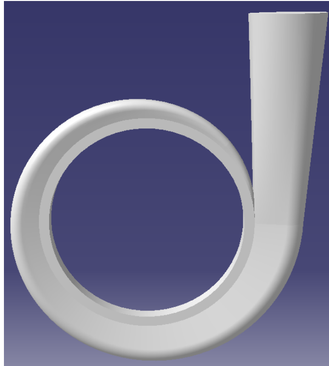
Figure 2. Unstructured designed volute by using Catia
