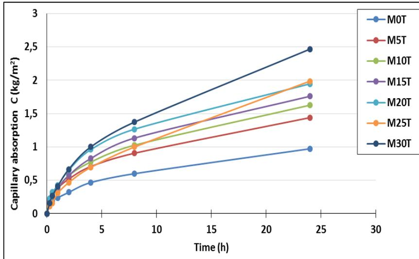
Figure 6. Evolution of the capillary absorption coefficient at 14 days of age.
