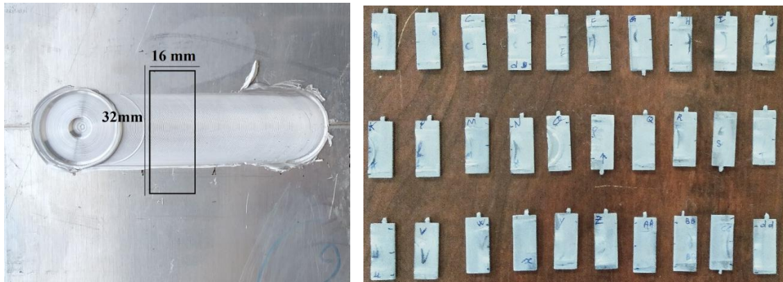
Figure 2. Cutting of specimens
