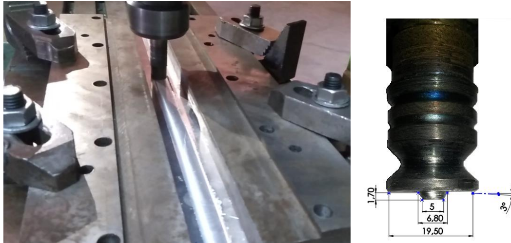
Figure 1. FSW process and the tool geometry
