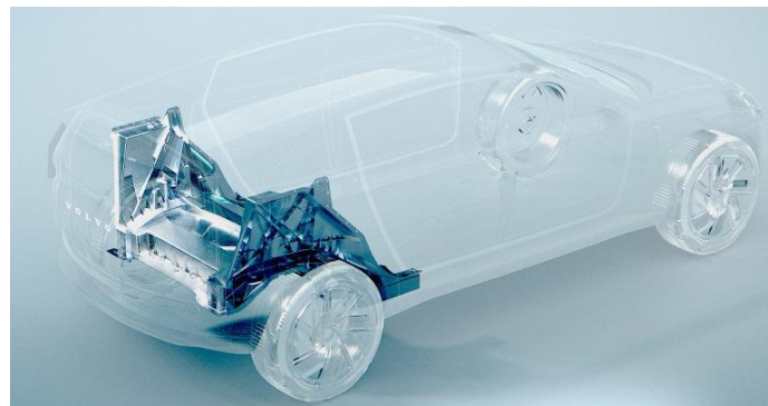
Figure 8. The megacasting replaces many stamped parts at the rear of this Volvo's chassis (Carney, 2022).
