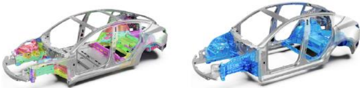
Figure 7. Production of Tesla Model 3 is revealed Tesla model Y by mega-giga casting technology (Duckers, 2022).
