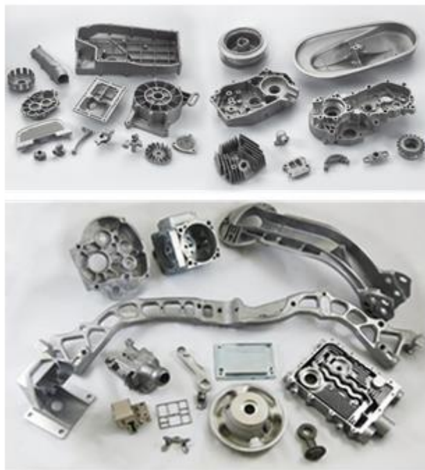
Figure 3. Examples of aluminum die casting components (Cheşa, 2019).
