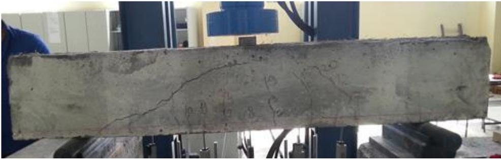
Figure 4. Crack pattern of B2.5P1.0
