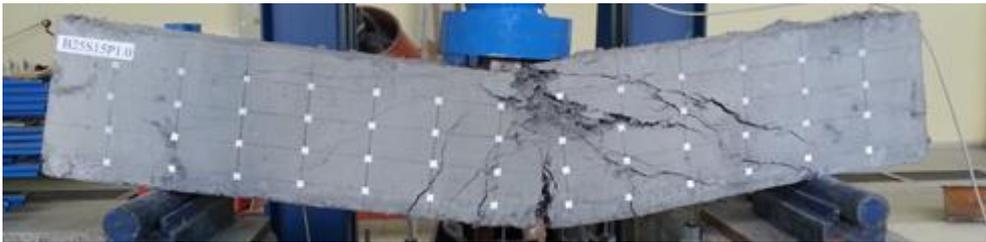
Figure 6. Crack pattern of B2.5S15P1.0
