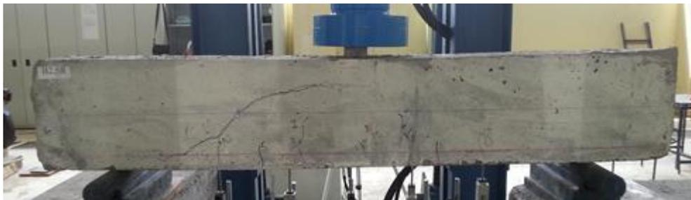
Figure 3. Crack pattern of B2.5R
