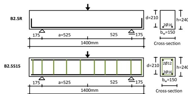
Figure 1. Geometry and reinforcement arrangement of beams
