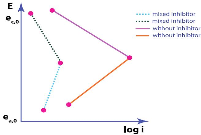
Figure 5. Mixed inhibitors are organic compounds (contain nitrogen and sulphur)
