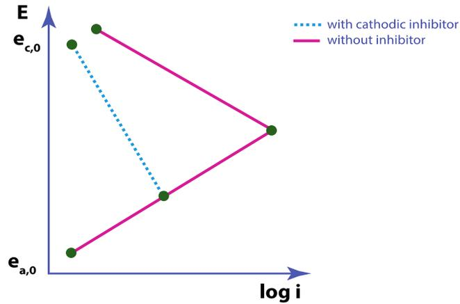
Figure 4. Cathodic inhibitors: calcium bicarbonate (Ca(HO<sub>3</sub>)<sub>2</sub>), Antimon (Sb<sup>3+</sup>), (on iron)
