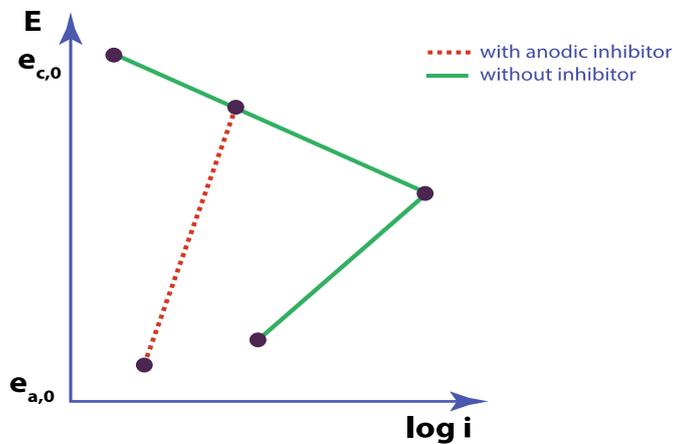
Fig 3. Anodic inhibitors: chromate ( $CrO_4^-$ ), molybdate ( $MoO_4^-$ ), benzoate ( $C_7H_5O_2^-$ ), silicate ( $SiO_4^{4-}$ )
