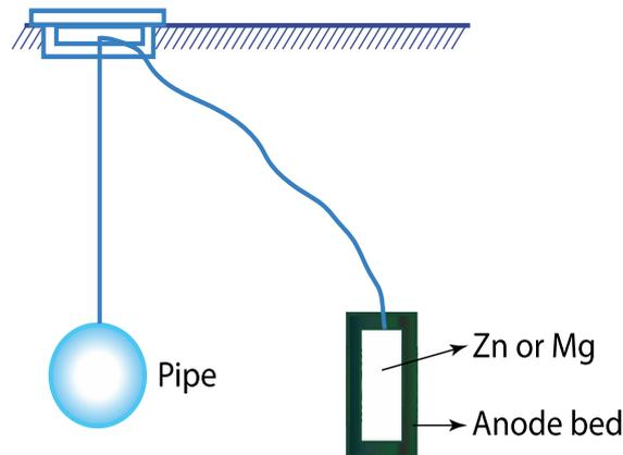
Fig 2. Cathodic protection of buried pipe helping anode bed.
