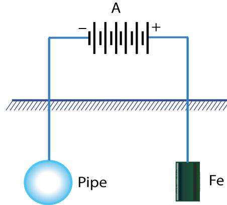
Fig 1. Cathodic protection with applied external source.
