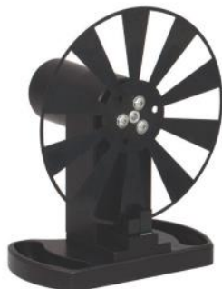
Figure 2. Head and wheel of the mechanical optical chopper
