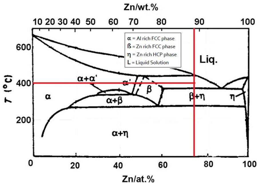
Figure 1. Al-Zn phase diagram
