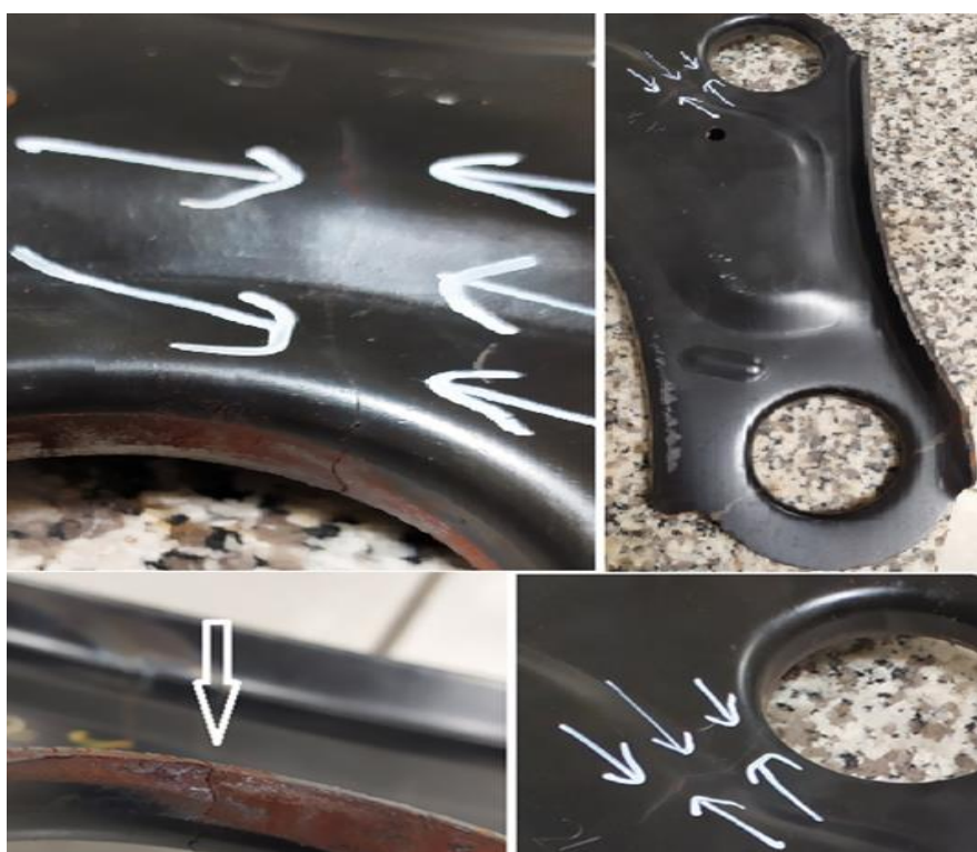
Figure 6. Crack regions on the cathaphoresis coated parts after fatigue test
