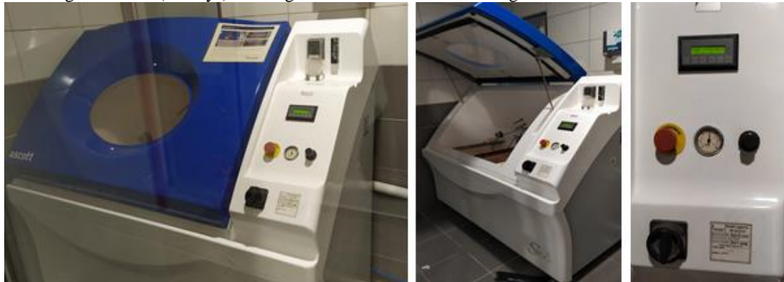
Figure 3. Ascott S450s brand salt spray corrosion test chamber
