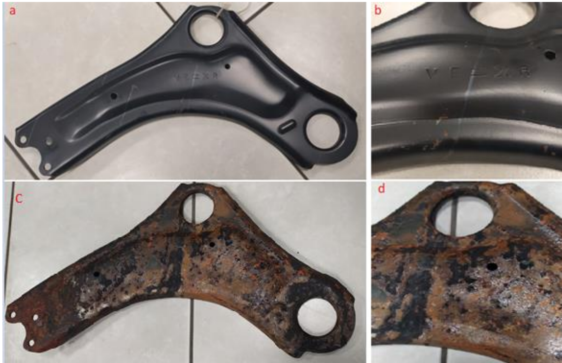
Figure 4. a,b) Cataphoresis coated control arm after 720 hours salt spray test, c,d) Uncoated control arm after 720 hours salt spray test
