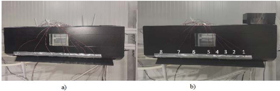
Figure 3. Comparative PTC laboratory tests a) without fresh air module b) with fresh air module
