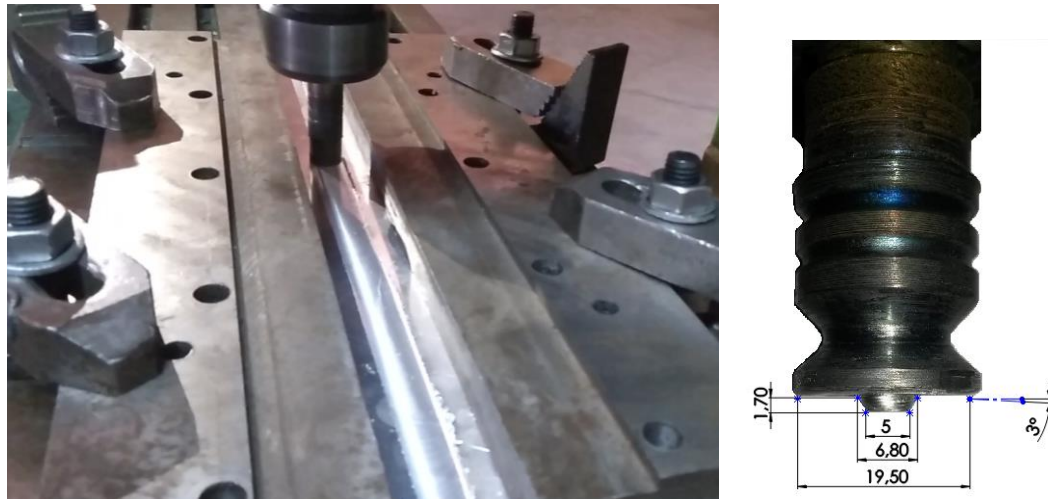
Figure 1. FSW process and the tool geometry
