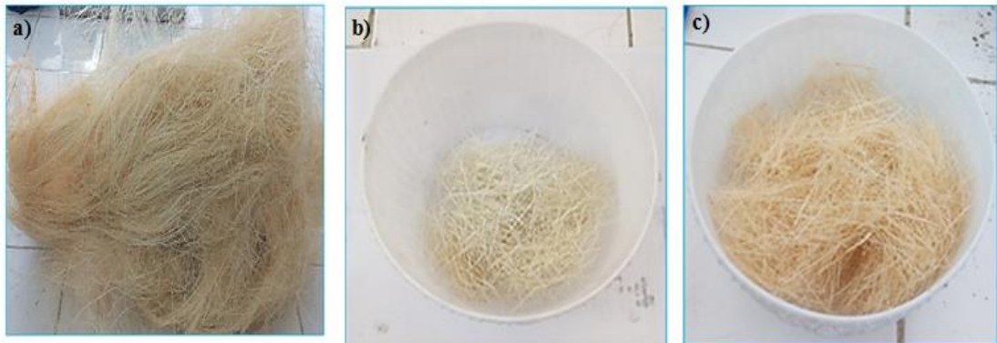
Figure 1. a) Sisal fiber, b) length sisal fiber 7cm, c) length sisal fiber 10cm.
