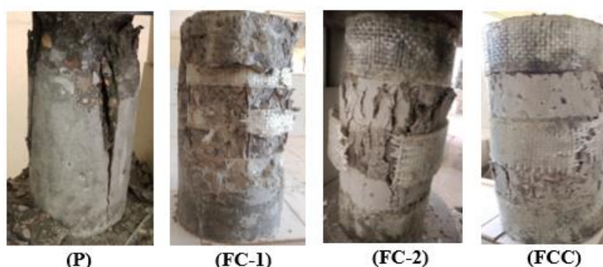
Figure 7. The modes of failure in the concrete column
