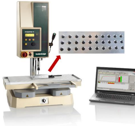
Figure 1. Tapping torque test system
