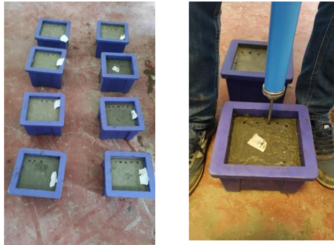
Figure 2. Determination of the initial and final setting times of specimens with penetrometer
