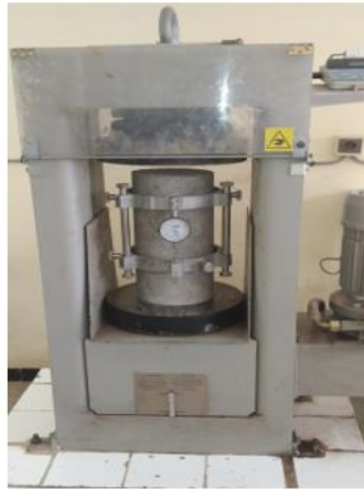
Figure 4. Axial compression loading set-up
