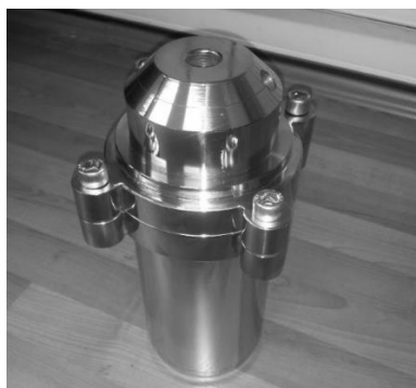
Figure 4. Fabricated vessel with hatch and clamps
