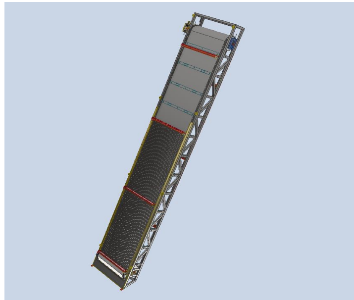
Figure 1. 3D modeling of mechanical bar screen
