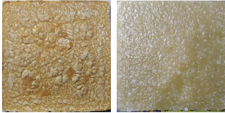
Figure 2. Photographs of the 40% lauric and paraffin composites
