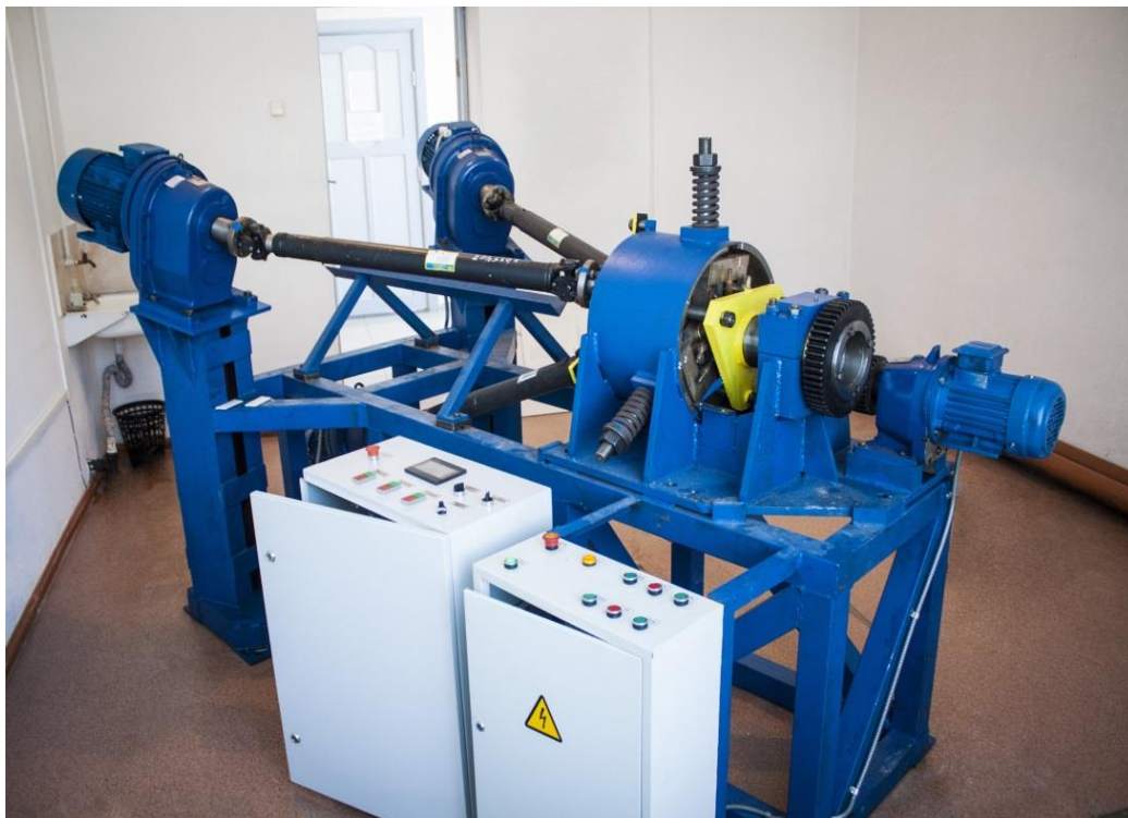
Figure 1. SVP-08 radial-shear rolling mill
