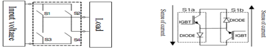
Figure 4. SPMC Structure, bidirectional switch module (Abrous, 2008)
