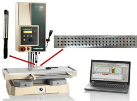
Figure 1. Tapping Torque Test System
