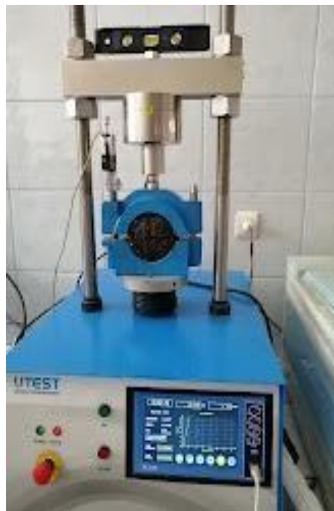
Figure 4. Performing Marshall stability and flow test
