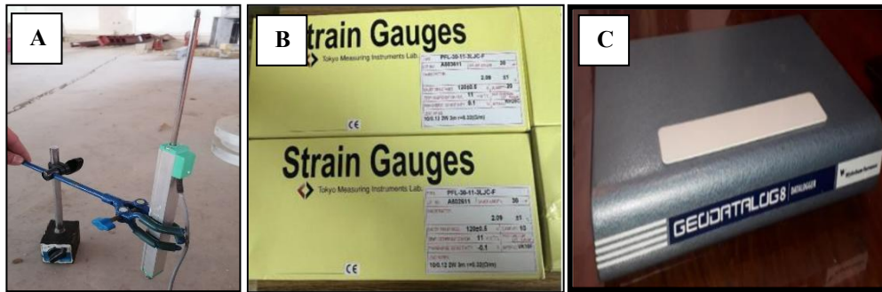
Figure 5. Devices of the test : A) LVDT, B) Strain gauges, and C) Data logger.
