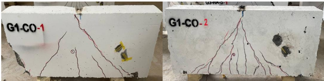
Figure 7. Failure modes of the control beams (G1)
