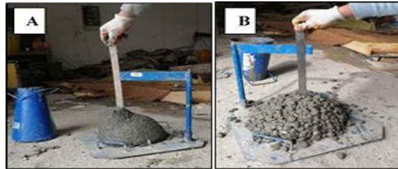
Figure 3. Slump test for A) HSC and B) NSC.
