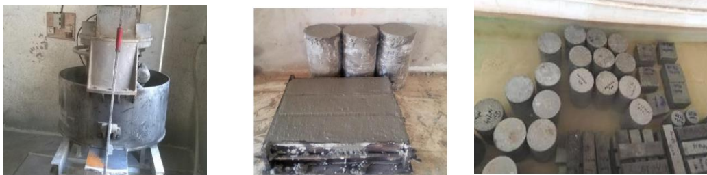
Figure 4. Casting and curing test specimens
