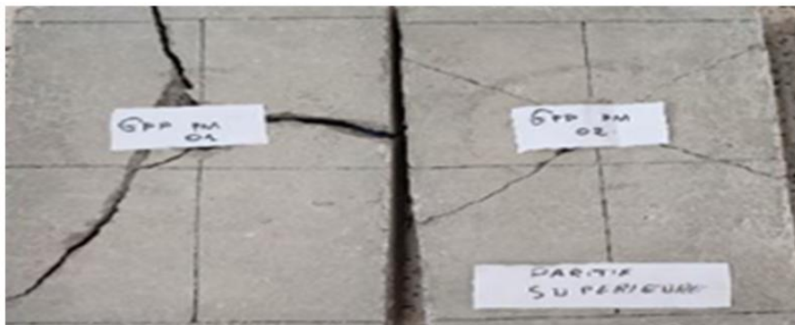
Figure 9. Example of failure mode of slabs reinforced by propylene fibers (series 2)
