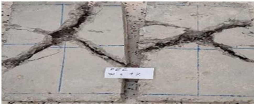
Figure 7. Example of failure mode of slabs reinforced by metal fibers (MF) (series1)
