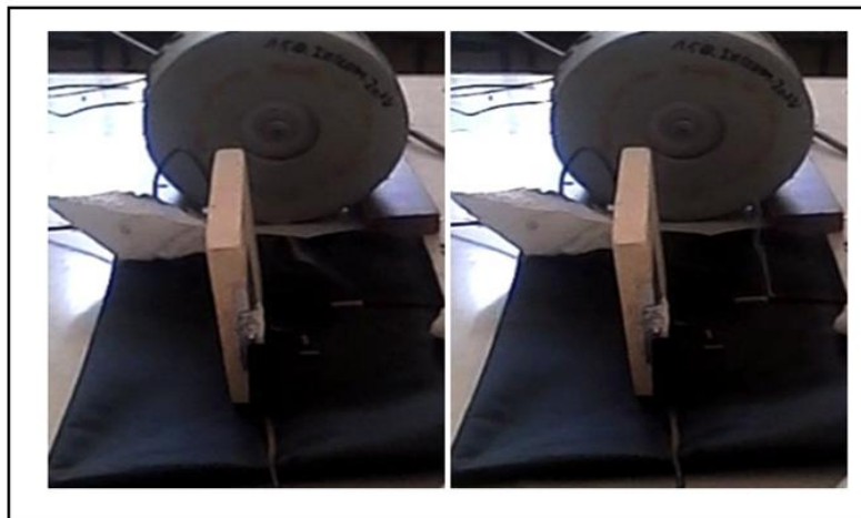
Figure 7. Observation of the smoke deflection angle for a frequency of 500Hz.
