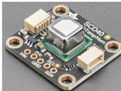
Figure 7. The electronic board on SDC40 CO2 sensor
